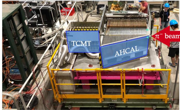
**Figure 5.3.:** The design of the AHCAL prototype and the TCMT for the test beam run at CERN in 2018 [50].
