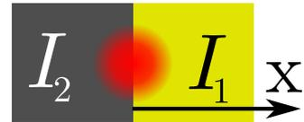
**Figure A.1.:** Beam is moved along a sharp edge to determine the beamwaist.
