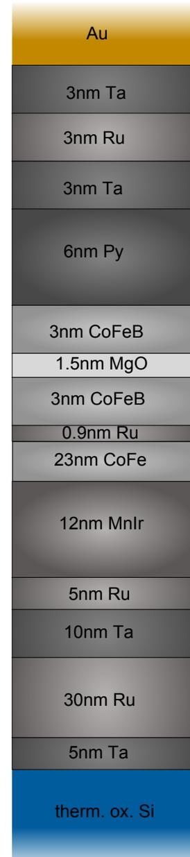
**Figure 4.11.:** Stack structure of the sample K120531a.
