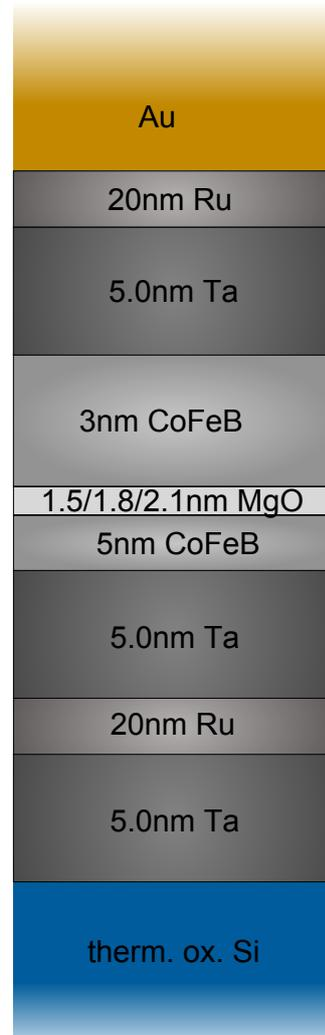
**Figure 4.3.:** Stack structure of the sample vd120111-x.
