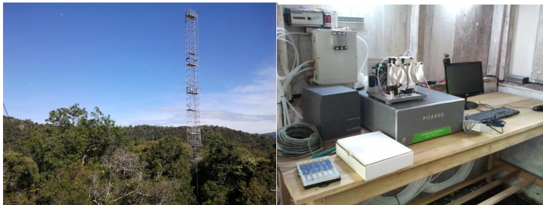
Bariri 70 m carbon flux tower and stable water vapour analyzer with calibration system.
